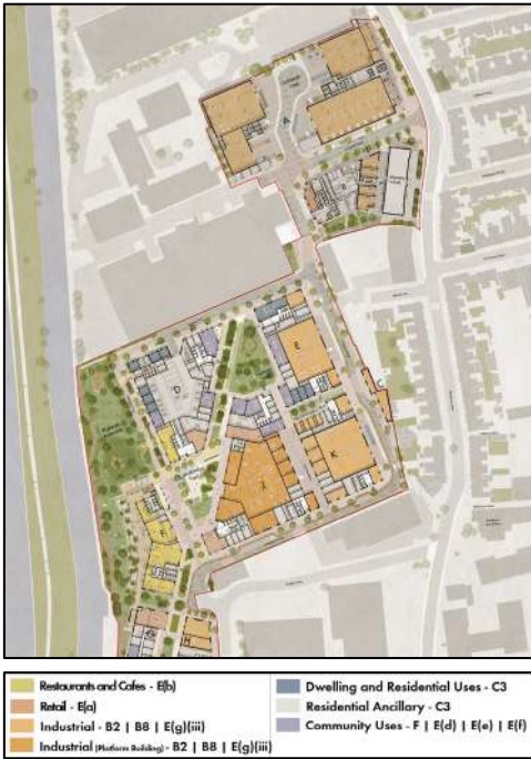
Figure 13: Proposed ground floor uses plan for Uplands Business Park, illustrating the spatial separation of industrial and residential uses on the site (Source: Allies and Morrison)
